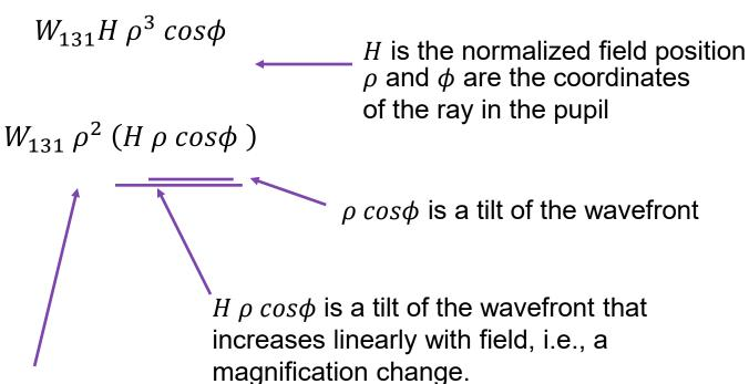
The  $\rho^2$  term means that the magnification change increases quadratically with the radial position in the pupil.
