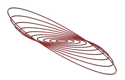
A series of concentric but increasingly tilted circles generates a comatic wavefront.
