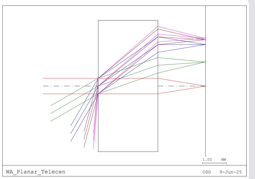
• A metalens covering a semi-field of 85° at F/3.
